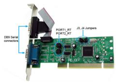
The two sets of jumpers on this card (J4, J3 and PORT1\_RT, PORT2\_RT) are used to configure the operating mode/serial protocol and 2/4-wire operation respectively.
